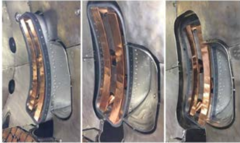
Fig. 3: The ICRH antenna at three radial positions inside the vacuum vessel of W7-X. Left: inside the plasma vessel, during ICRH operations; middle: as part of the first wall of W7-X during plasma operations without ICRH; right: inside the ICRH port.
