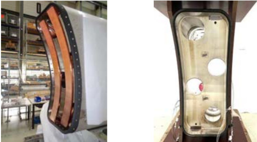
Fig. 7: The ICRH antenna after the first high power commissioning on W7-X plasma's. Only a slight discoloration could be seen in the antenna box.
